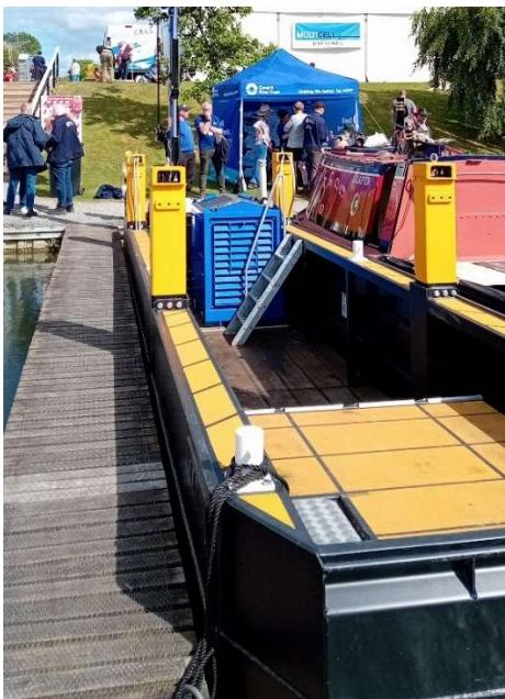
A new work-boat commissioned by CRT with its own power supply for hydraulic feet and a platform for a tracked dredging machine was shown off at the Crick Boat Show this year...
