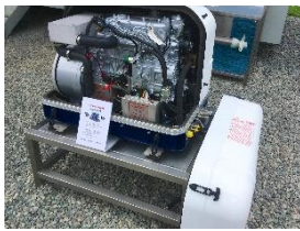
A Typical Marinised Diesel Generator
