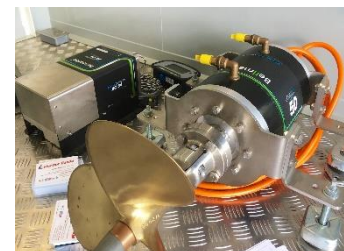
A Typical PMAC Motor With Control Gear
