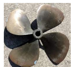
A Typical Four Bladed Propeller
