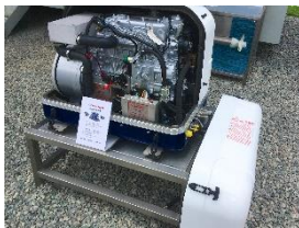
A Typical Marinised Diesel Generator
