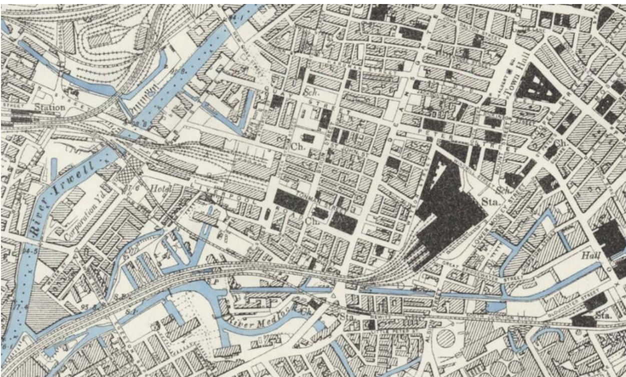
Figure 2.2 1875-1899: The Manchester & Salford Junction Canal after the through route was severed in 1875. Locks No.3 & 4, the reservoir and upper pump house have been replaced by Manchester Central Station. OS 6" Series Map 1894 (published 1896).
