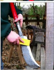
Hold the tool with the blade away from you; try to hold the sharpening stone at the same angle as the blade.
