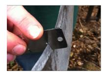
Use the gauge provided to check the blade angle.
